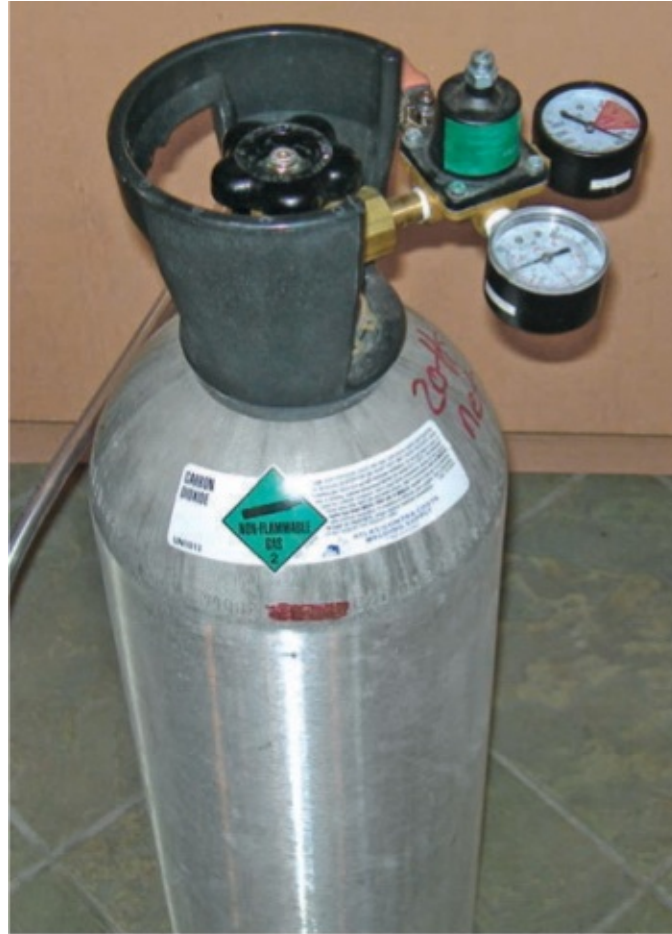
A 20 lb (9 kg) aluminum tank weighs about 35 lbs (16 kg).
